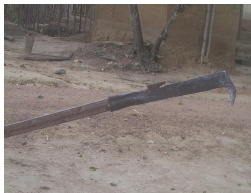
Cutting head of Harvesting Hook
